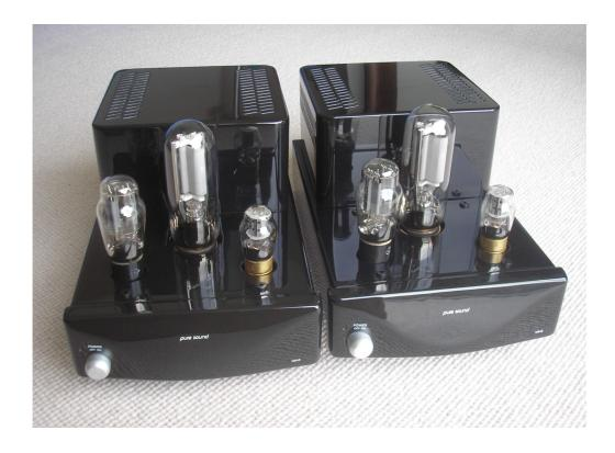
The M845 mono power amplifier is a single ended design based around the 845 power triode. Operating in Class A and giving 27 Watts of output power, it will complement a wide range of medium to high efficiency loudspeakers.
