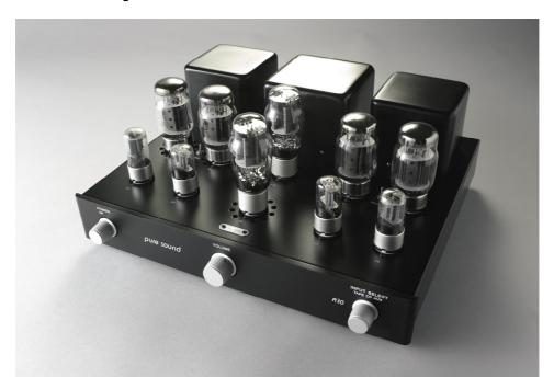
The amplifier uses the very robust Electro Harmonix 6550 output valves in an Ultra Linear Push Pull configuration. This arrangement gives a combination of power and clarity that is difficult to beat. The amplifier uses an Auto Bias system, which means that replacement output valves should be fitted as matched pairs. There will be no need to reset or monitor bias conditions.
